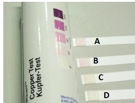
Figure 14A. Copper Test, Cleaning Agent C – Trial 26: No Reflow, 6 passes
