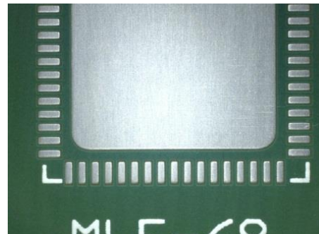
Figure 8D. Visual Inspection, Cleaning Agent D – Trial 40: Reflow, 6 Passes
