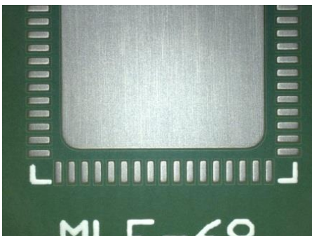
Figure 10B. Visual Inspection, Cleaning Agent A – Trial 12: Reflow, 6 Passes
