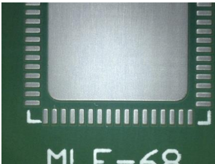
Figure 8A. Visual Inspection, Cleaning Agent C – Trial 26: No Reflow, 6 Passes
