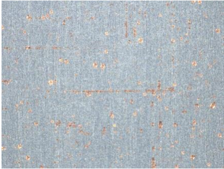
Figure 7B. Visual Inspection, Cleaning Agent A – Trial 4: Reflow, 6 Passes
