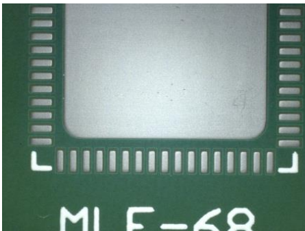
Figure 10A. Visual Inspection, Cleaning Agent A – Trial 10: No Reflow, 6 Passes
