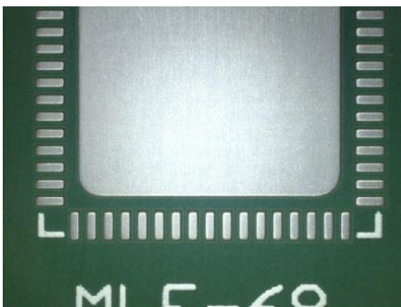
Figure 8B. Visual Inspection, Cleaning Agent C – Trial 28: Reflow, 6 Passes
