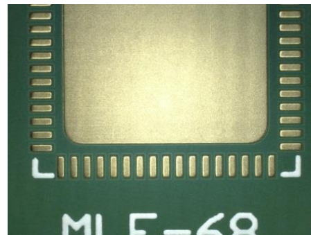
Figure 11A. Visual Inspection, Cleaning Agent A – Trial 6: No Reflow, 6 Passes
